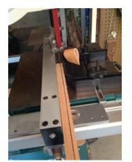
With the width wedges cut off, I marked the cut edges of the limbs to 1/2" thickness, and put them back on the band saw. After first making a couple of stop cuts at the ends of the handle area, I set up a fence and ran the limbs through until reaching the stop cuts.
