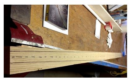
The design we'll use this year is a "pyramid" bow, which our Dave Martin has explored in some detail. The idea of the pyramid is that if the width changes enough from the handle area to the tips, the bow will bend nicely without having to do much thickness tapering.
