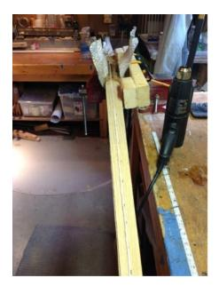
Here's the same stave after coating the center section with vegetable oil, to prevent burning and to carry heat into the wood. Using the heat gun (around 1350 degrees F) we get the wood too hot to touch without scorching.
