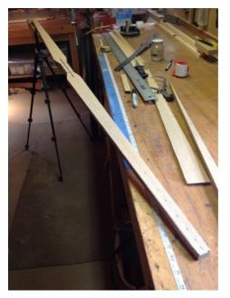
This starts to look like a bow, but clamping a test cord between the tip centers clearly shows that they don't line up with the center of the handle.
