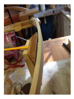
Here's the "tillering gizmo" held up against the belly of our oak pyramid example bow. The pencil is screwed into a nut in the gizmo, and extends just slightly from its base.
