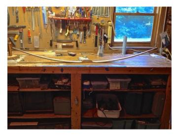
At this point, you have a stave braced at close to normal height. If you've been paying attention, you've corrected any major problems. Both limbs should be bending approximately the same, with the "tiller" or measurement between the string and the limbs some distance from the center approximately the same - let's say within 1/2 - 3/4".
