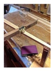
It is important not to become fixated on one limb - remember that each change you make in any one place will show up as a different bend everywhere along the bow. Here's one limb (at right) that was worked on a bit too much, before I noticed how much the bend on the left was reduced. I had to reduce the left limb to match, resulting in a pretty but underweight bow.
