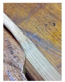
breaking loose from the limbs at the stress point. If all goes well, this will strengthen the stress point and make the limbs bend more farther away from the center - a bit more sanding midlimb should also help reduce stress inboard at the cost a a pound or two more draw. I was at 42# before the tweaking began, we'll soon see if all this work gained anything.
