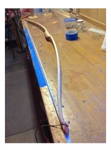
I can certainly attest that with these changes, the bow was a whole lot harder to brace than before. As usual, I did 20-30 pulls before putting the bow on the scale. At 15" of draw, it pulled about 23#, 2-3# more than earlier. A rule of thumb tells us that the draw at 28# is usually about twice the draw at 15", so this suggests a final draw weight of 45-47#, a bit less than expected.
