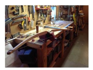
Working through these steps patiently will get you to the point shown at right - here's our pyramid bow at 5.5" brace height. Checking the limbs for "tiller" (bowyers use that word a lot) is done by measuring the distance from the string to each limb, the same distance from center, I use 12".
