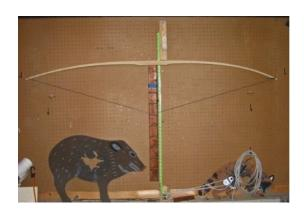
Another, less dramatic example at left: this one is slightly better but still shows significant differences between the stiffer left limb and the weaker right limb. It needs wood removed from the left mid-limb until at this same amount of pull, both limbs bend the same.
