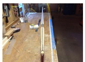
Here is another bow at its first "low brace". We've adjusted the bowyer's knot in our long string using to provide about 3" of brace height (between string and the handle, where your hand grips it). This may be 1"-2" shorter than your nock-to-nock length. Because the low brace leaves the limbs almost straight, it isn't putting nearly as much strain on them as a normal brace will.
