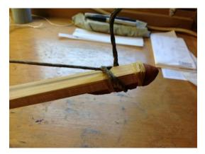
To go beyond floor tillering, we need something on the limb tips to hold a string. To reduce stress on the new bow, we start with a "long string", so that the bow is not under tension except when drawn.
