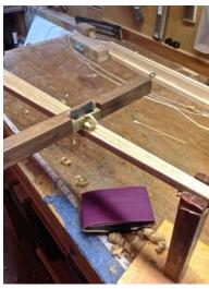
Here's what we have at this point. The tips and handle are nicely lined up, but as a result of our heat-bending, the tips are "deflexed" (bent back in the "draw" direction) slightly. This is not a problem, as it was caused while bending the handle - not by a breakdown in wood resiliency called "set" caused by over stressing one particular section of wood. We'll be watching for this "set" while we tiller the bow, by checking how far the tips at rest have moved back from where they started.
