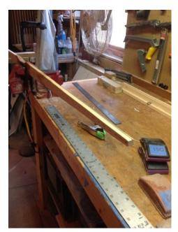
First, I trimmed the pyramid profile from the widest part of the limb straight to 1/2" tips, 1/4" on either side of a straight line from tip to tip through the handle center. I did this with the band saw, but you can easily do it with a hand plane, rasp, or sanding block. We'll cover use of hand tools on bows during the clinic.
